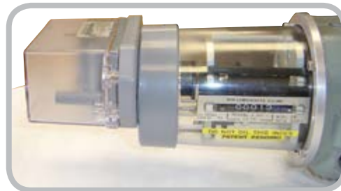
AMR Adapter and ERT installed on a Dresser meter (top inlet meter installation shown)
